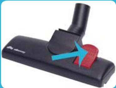
**EN:** Use the floor/carpet nozzle for hard floor surfaces with the brush of the nozzle extended, and for carpets with the brush withdrawn. Change the position of the brush with the button located on top of the nozzle.
